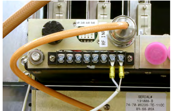
Figure 2B: The ACM power cable connected.
